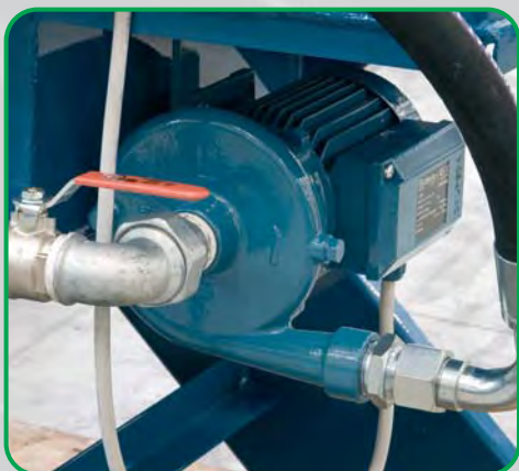
Oil circulation electric pump with cut-off valve (ORVS 3, 7, 14 excluded)
